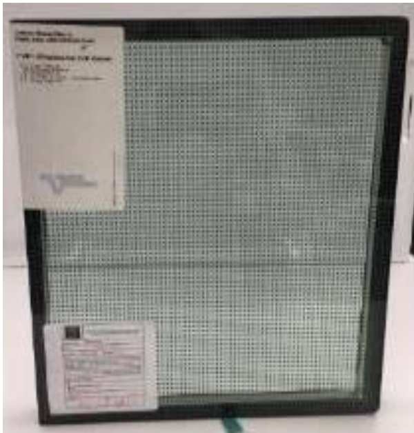
Figure 6. Examples of Ceramic Frit Patterns on glass with a TF of less than 25 at locations shown in Figure 4 and 5, respectively (Source: FXCollaborative)
