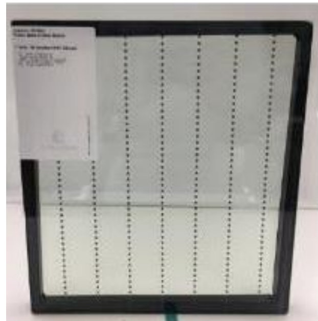
Figure 6. Examples of Ceramic Frit Patterns on glass with a TF of less than 25 at locations shown in Figure 4 and 5, respectively (Source: FXCollaborative)
